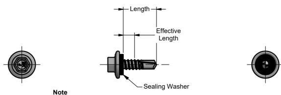
Lengths from underside of sealing washer and includes compression.
