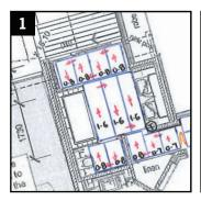
**Plan out the installation** Determine the location of the Thermostat and floor sensor and work out the layout of the heating mat excluding areas under floor mounted fixtures.
