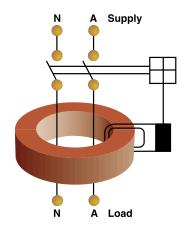
During normal operation, these Active and Neutral currents are in balance. However, should any current flow to earth, an imbalance is sufficient (30mA), the 2025RC will cut the electrical supply in less than 40 milliseconds, perhaps the most important fraction of a second in someone's life.
