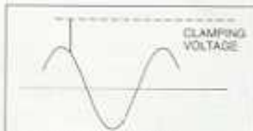
SPIKE SAFELY CLAMPED
