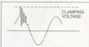
TRANSIENT SAFELY CLAMPED
