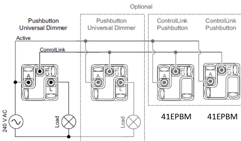
Wiring Diagram – for Multiway dimming
