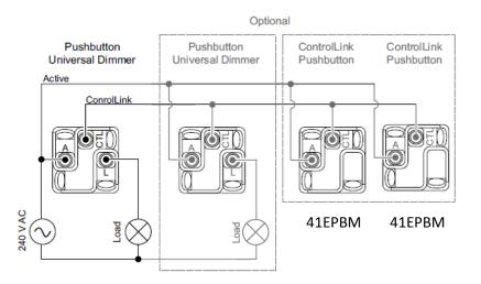
Wiring Diagram – for Multiway dimming
