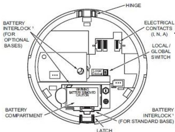
NOTE - Local/Global Switch - defines the relay trigger function on the optional 755RB relay base only.
