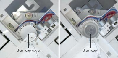
Remove drain cap cover and check the condition. If it is necessary to clean-up, firstly remove the rubber plug to drain water out and secondly remove the drain cap.
