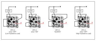
Note: Low Impedance Load examples include incandescent, halogen, resistive loads.
