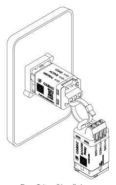
Figure 5: In wall installation.
