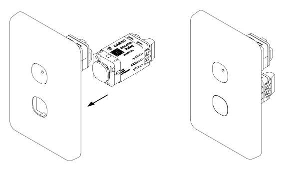
Figure 4: Wall plate installation.
