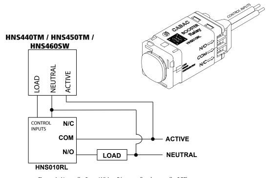
Figure 1: Normally Open Wiring Diagram (load normally OFF)
