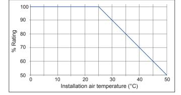
Note: Operation at temperature, voltage or load outside of the above specifications may cause permanent damage to the unit. When used in ambient temperatures above 25°C the timer must be de-rated according to the chart.
