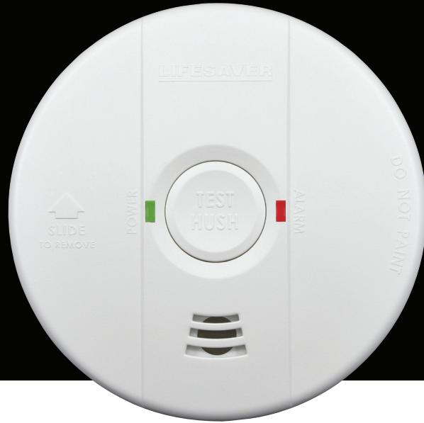
The PSA Lifesaver 6800RL model is a mains powered, rechargeable lithium battery backed smoke alarm. The alarm uses photoelectric technology and is designed to be surface mounted on the ceiling or wall. It can be used as a single stand alone unit, or can be interconnected with up to 24 units.
