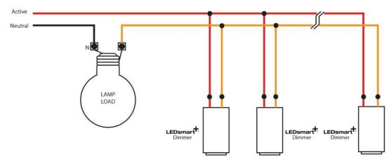
Three-way dimming and switching using **LEDsmart**<sup>+</sup> dimmers. Note that each two-wire **LEDsmart**<sup>+</sup> dimmer is simply wired in parallel.
