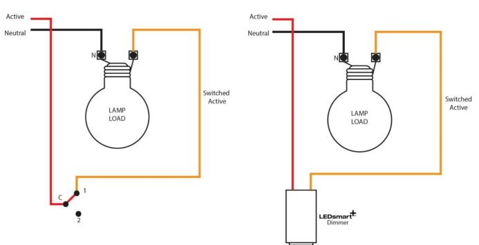
**Replacement one way dimming/switching**
