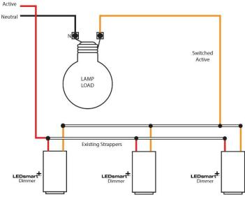
Traditional three-way switching using two rocker switches and one intermediate switch, with strappers between the switches. Rocker switches and intermediate switch replaced with LEDsmart<sup>+</sup> dimmers. The existing strappers are used to connect the dimmers in parallel. No new wiring is required.
