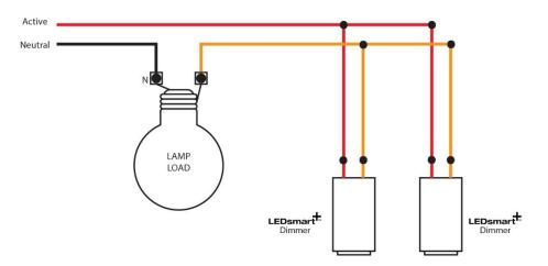
Two-way dimming and switching using LEDsmart<sup>+</sup> dimmers. Note the two-wire dimmers are simply wired in parallel.
