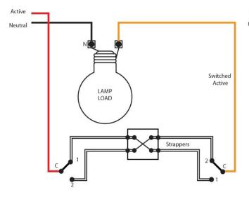
Replacement three-way dimming/switching
