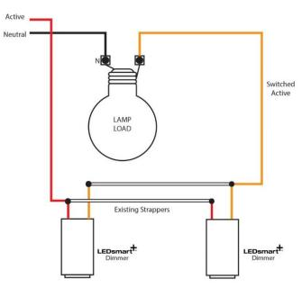
Traditional two-way switching using standard rocker switch mechanisms and strappers between the switches.
