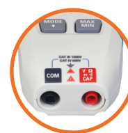
Rear entry of standard 4mm Test Lead Terminals
