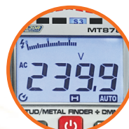
4000 Count Backlit LCD with 41 Segment Bargraph
