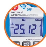
4000 Count Backlit LCD Display
