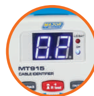
Receiver Two Digit Blue LED Display
