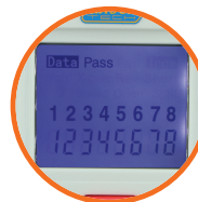
Backlit LCD display maps out visual representation of cable
