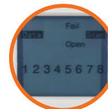
Backlit LCD maps out connections & describes wiring faults
