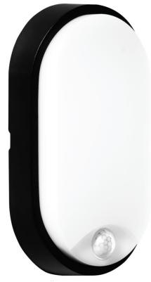
PIR Sensor: Detection distance 8m max. (<22°C) Ambient light <10LUX ~ 2000LUX (adjustable) Turn on-Time 10S±5S ~ 5min±1min (adjustable)
