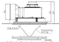
Figure 1: Installing ducting (sold separately)
