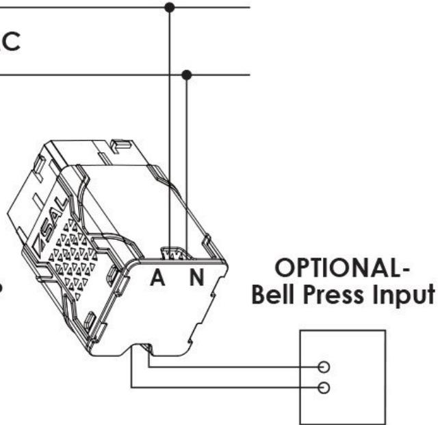
There is no polarity on the bell press conductors.
