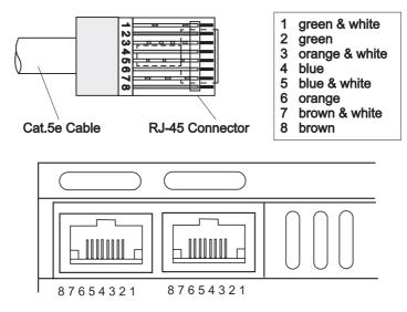
Figure 2. C-Bus network connection
