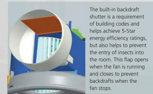
The built-in backdraft shutter is a requirement of building codes and helps achieve 5-Star energy efficiency ratings, but also helps to prevent the entry of insects into the room. This flap opens when the fan is running and closes to prevent backdrafts when the fan stops.
