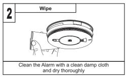
Use the narrow nozzle attachment of your vacuum cleaner to remove dust, insects and cobwebs from the sides and cover slots where the airflow enters. Clean the outside cover by occasionally wiping with a clean damp cloth then dry thoroughly with a lint free cloth. Do not use any cleaning agents, bleaches, detergents or polishes, including those in aerosol cans.
