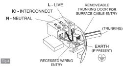
There are two other positions which are also suitable for the surface wiring to enter (and exit) the alarm, one next to the removable section and another directly opposite.
