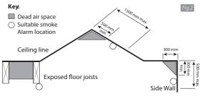
DEAD AIRSPACE AND PROPER MOUNTING OF SMOKE ALARMS ON SIDE WALLS
