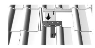
3. The roof hook must not press against the roof tile. If necessary, shim the roof hook with wood.
