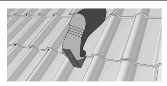
6. Variation for installation on plain tile roofs with plain tile roof cladding, a recess must be cut into the tiles around the position of the roof hook.
