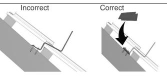
4. If necessary, use an angle grinder or hammer to cut a recess in the tile that covers the roof hook at the point where the roof hook comes through so that the tile lies flat on the surface. If grooved tiles are used, it will also be necessary to cut a recess in the lower tile. For high profile (Spanish) tiles a Roof Hook Extender can be used.
