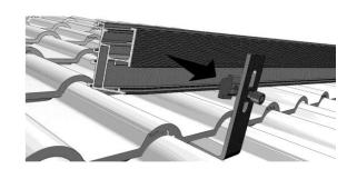
9. Adjust to necessary vertical and horizontal position by using the slot hole in the roof hooks and connection of the Z-Module or on the rail.
