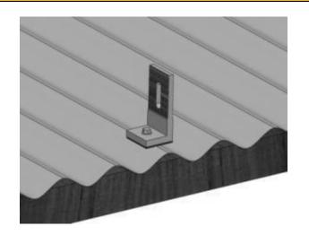
9.2. Place the supplied EPDM rubber under the L-Feet in the way that the screw goes through the hole in the EPDM rubber pad. When fastening the screw make it sure that you don't deform the corrugation of the roof cladding. This can happen if you penetrate too deep with the screw when fastening.
