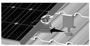
20. Now slide in the first module of the next row from above onto the corresponding PV module of the row beneath. A separation from the lower module can be maintained for optical reasons. An inter-module clamp can be used as a separator, so that the vertical and horizontal separation of the modules is identical. Continue mounting the PV-Modules as described in steps 15 to 20 until all PV modules are installed.
