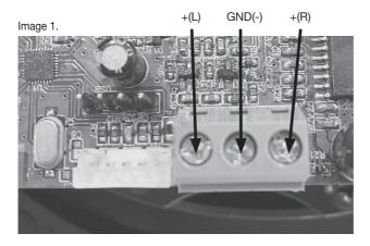
Image below shows example of a fixed wall connection link to the AUX terminals:
