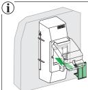
Note: Use pole filler provided in accessory bag to fill the empty modules before closing the cover.
