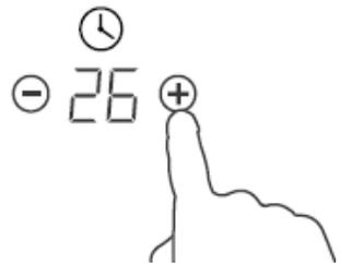
If the setting time exceeds 99 minutes, the timer will automatically return to the minute 0.
