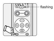
4. Your RS10 remote should now be ready for use. Check for correct operation of the remote. If it is not working correctly repeat steps 2~4 until correct code is located.
