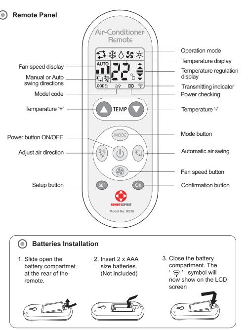
1. Turn on the power to your air condi tioner at the main unit. Then point the RS10 controller at the unit.
