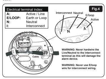
Refer to the manual for more details on the correct circuit wiring.
