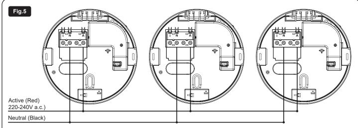
**Note:** Never have hard wire interconnection with multiple RWB bases. Multiple RWB bases must be connected through RF. RWB interconnect terminal is only for connection directly to other smoke alarms and/or heat alarms.
