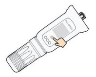
figure 7-1 Enabling the WLAN Hotspot
