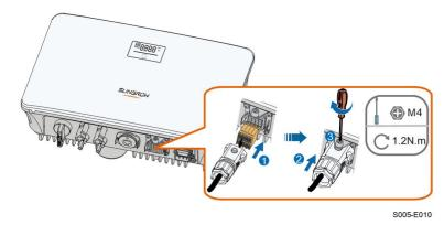
step 7 Slightly pull out the cable and then fasten the swivel nut. Lock the connector with the screw.
