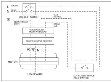
**Step 1:** Connect the EARTH wire to the terminal port marked <sup>\*</sup> on the terminal block mounting bracket.
