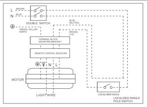
Step 1: Connect the EARTH wire to the terminal port marked "
