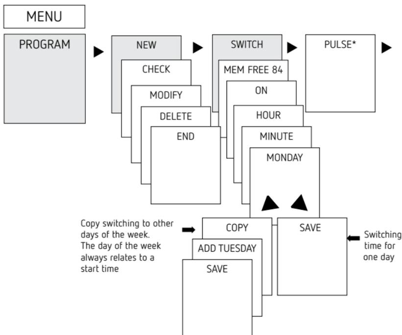
① A switching time always consists of a start time and an end time
