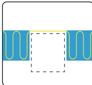
Remove the mesh to avoid permanent fixtures
