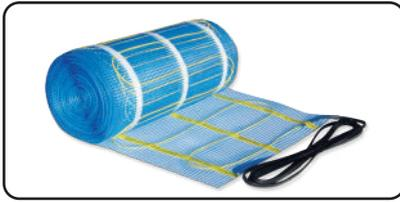
Thermonet is an underfloor heating mat system that is designed for installation beneath tiles or screeds. The system comprises of a 500mm wide self-adhesive mesh that holds the heating element in place, at the correct spacing and sticks down directly to the substrate.
