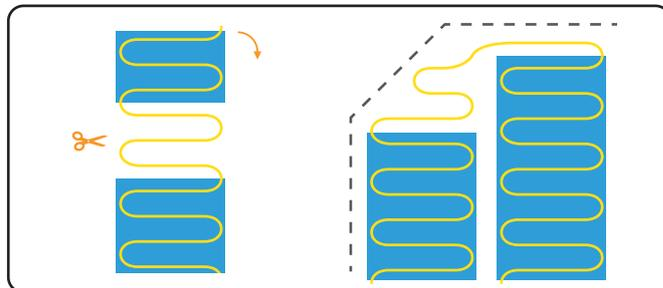
Remove the cable from the mesh and tape in place for awkward areas such as angled walls
