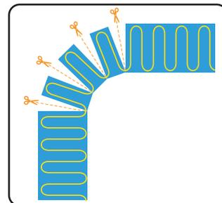
Cut the mesh into sections to make a curved fan turn
