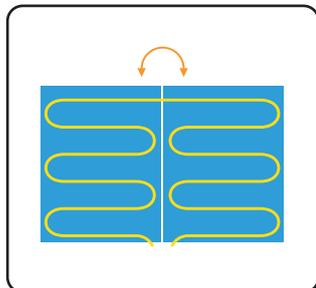
Turn the mat 180° laying the mat parallel to the first run
