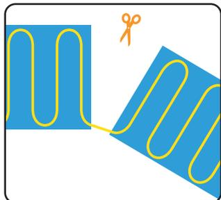
Use scissors to carefully cut the blue mesh – NEVER cut the yellow cable
