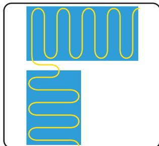
Release cable from the mat for an alternative 90° turn
