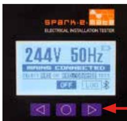
LOG button for sending test result to laptop
