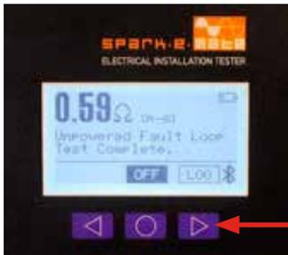
Press the LOG button to send result to your Android device
