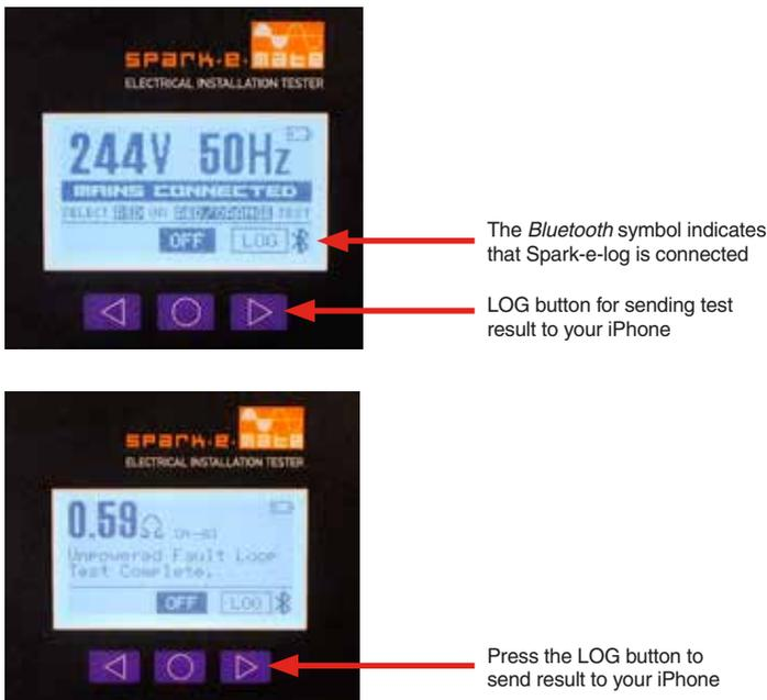
Both *Spark-e-mate* and your iPhone will “beep” to indicate successful data transfer. The test result appears in the Logs screen and is saved in Spark-e-log’s database.
