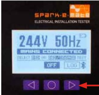
LOG button for sending test result to your Android device
