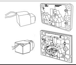
30USBCM with standard clip into twin socket 2025 / C2025.
