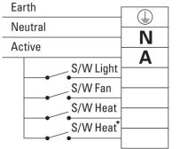
\*Second heat switch not required for model with 2 heat lamps
