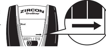
Continue sliding tool. When the center of a stud is located, three bars on the Signal Strength Indicator, the four Middle bars, CENTER display, and SpotLite® Pointing System will all illuminate and the buzzer will sound.
