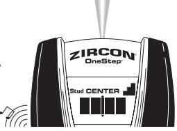
In cases of deeper studs (thicker walls), when the center of the stud is located only two bars will show on the Signal Strength Indicator and only the SpotLite® Pointing System and four Middle bars will illuminate. If you still cannot locate a stud, try STUD DEEPSCAN® mode. In STUD DEEPSCAN® mode, the Stud icon will continuously flash.
