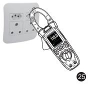
**Notes:** The detector is designed with high sensivity, static electricity and other sources of electrical energy may randomly activate the detector. This is normal operation, the detector only activates the indicator light when AC voltage is present, it does not indicate the voltage level on the LCD display.
