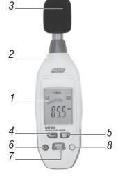
RANGE/(A/C) button: Press to switch range gear; hold to switch unit.
