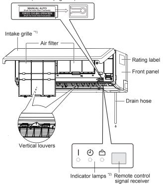
\*1) Before starting operation, make sure that the intake grille is closed completely. Incomplete closing may affect the proper function or performance of the product. \*2) Indicator lamps light in the following conditions.
