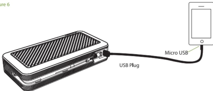
2. Turn on the USB charging by pressing the USB Power ON/OFF Button on the powerstation go rugged with air compressor.
