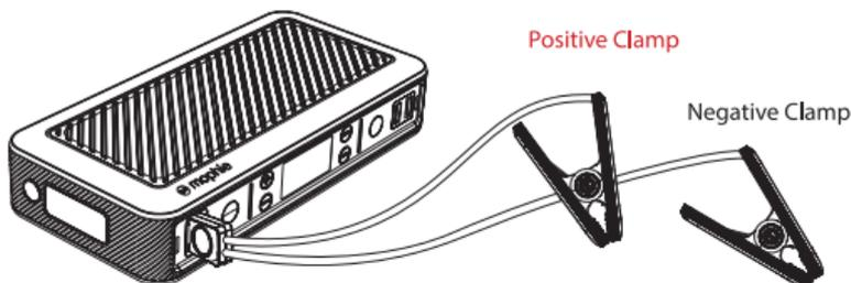
2. Attach the jumper cable clamps to the vehicle battery.
